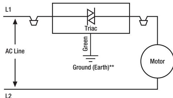
Connection Diagram for 3-Wire\* Controls (Switch Models)
