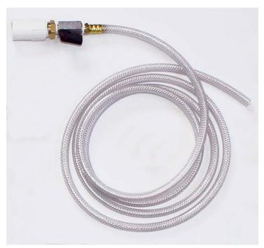
Turn on the misting system and adjust the Anti-Drip Valve to allow a slow trickle of water to escape. When you turn the misting system off, the water will continue to bleed off through the hose for a few seconds, but the nozzles should stop dripping very quickly. Adjust the valve until you are satisfied with the timing and amount of bleed-off.
